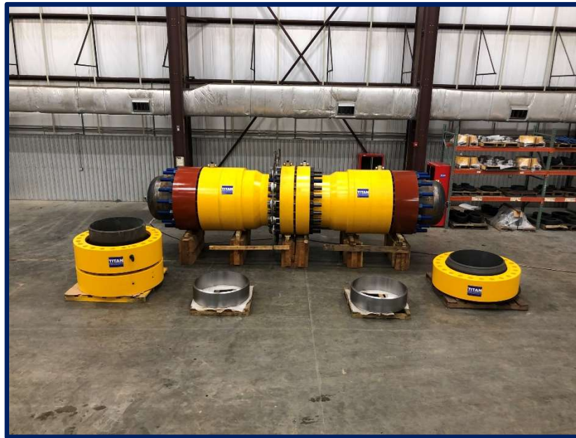
42" 3000psi Emergency Pipeline Repair System
